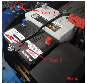
10. Fit Main/Cranking battery earth cable to captive nut on radiator support panel near bonnet buffer (Refer Pic 4.). Remove paint with scraper or file to ensure electrical contact. Spray over area with battery terminal protector once earth cable is secure.
