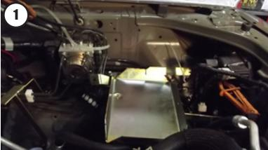
**4.** Fit short M6 bolts to captive behind headlight (behind indicator); beside headlight into existing hole, plus wizloc nut; on inner guard into existing hole, plus panel washer and wizloc nut. Long M6 bolt (from engine side) to angled arm low on radiator support panel with wizloc nut. Tighten all tray fixing bolts.
